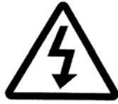
Danger!: High voltage
